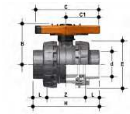
VXEIC Easyfit 2-way ball valve with female ends for solvent welding, metric series
