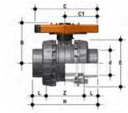
VXEAC Easyfit 2-way ball valve with female ends for solvent welding, ASTM series
