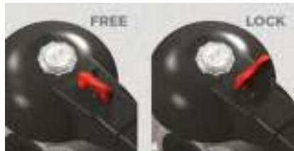
Thanks to the multifunctional handle and the red manoeuvre button on the lever, you can perform a 0°-90° operation and a graduated operation by means of the 10 intermediate positions and a stop lock: the handle can be locked in each of the 10 positions by simply pressing the Free-lock button. A lock can also be installed on the handle to protect the system against tampering. The valve is two-way and can be installed in any position. It can also be installed at end line or tank.
