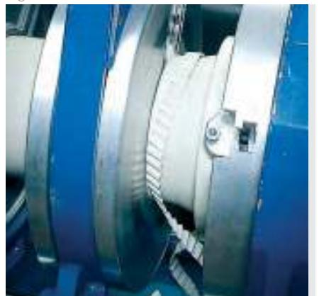
any traces of dust have settled on the planed surfaces, before they can be welded they should be cleaned with a cloth soaked in specific detergent.
