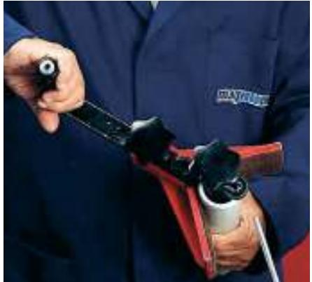
fering process can be performed either after peeling or concurrently with this operation, using special calibrated tools.
